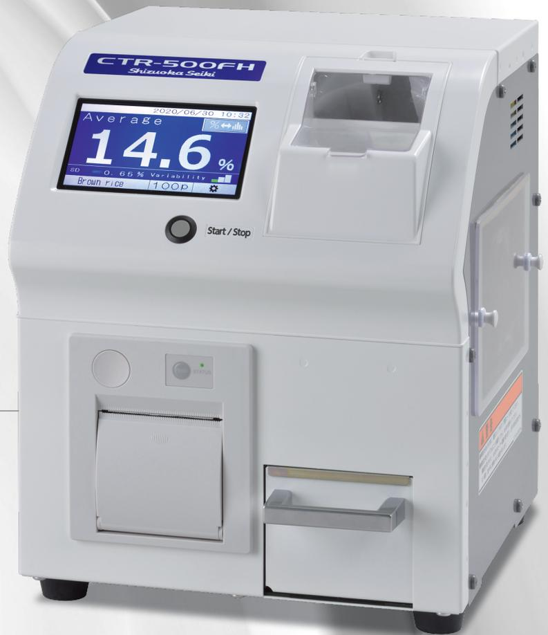
**Fast moisture distribution analysis at a time of receiving grains.**
